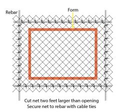
The Pour-In-Place Safety Net System is designed to secure open floor hazards with robust fall-through net protection. This effective safety net system safeguards workers from falls while containing materials, tools, and debris at floor level.
